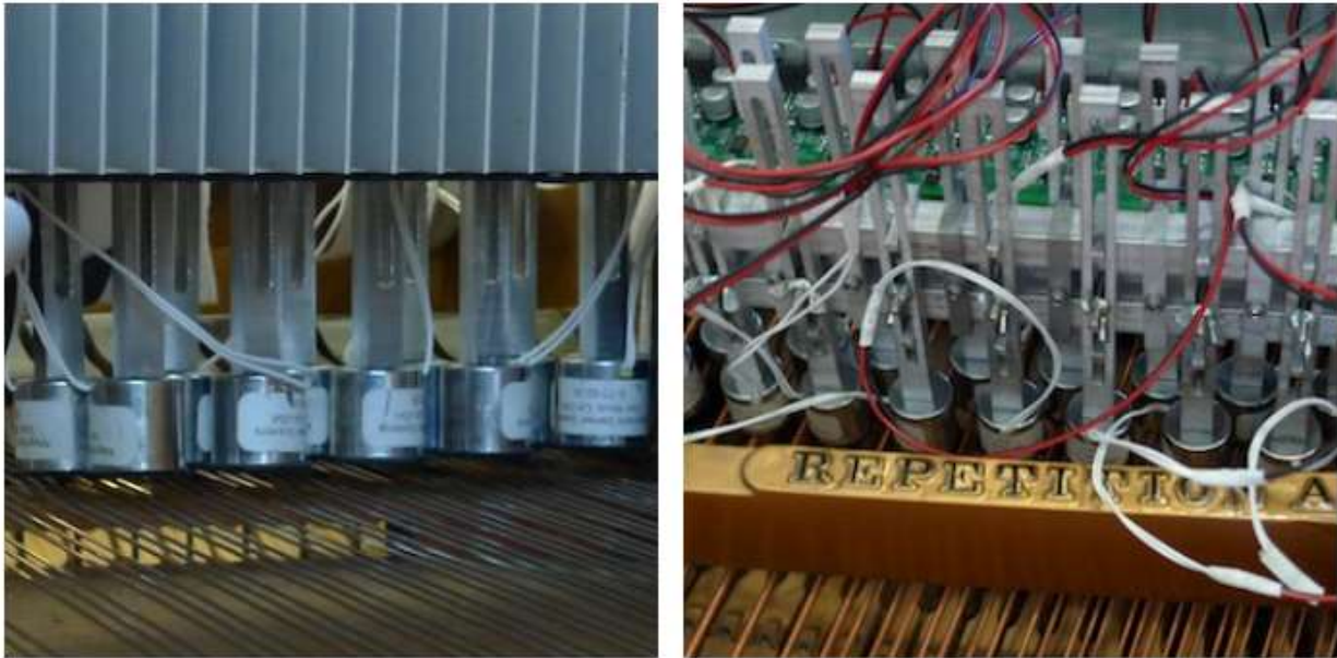
Figure 1. An electromagnetically prepared piano An elaborate set of holding electromagnets held over piano strings [4].
